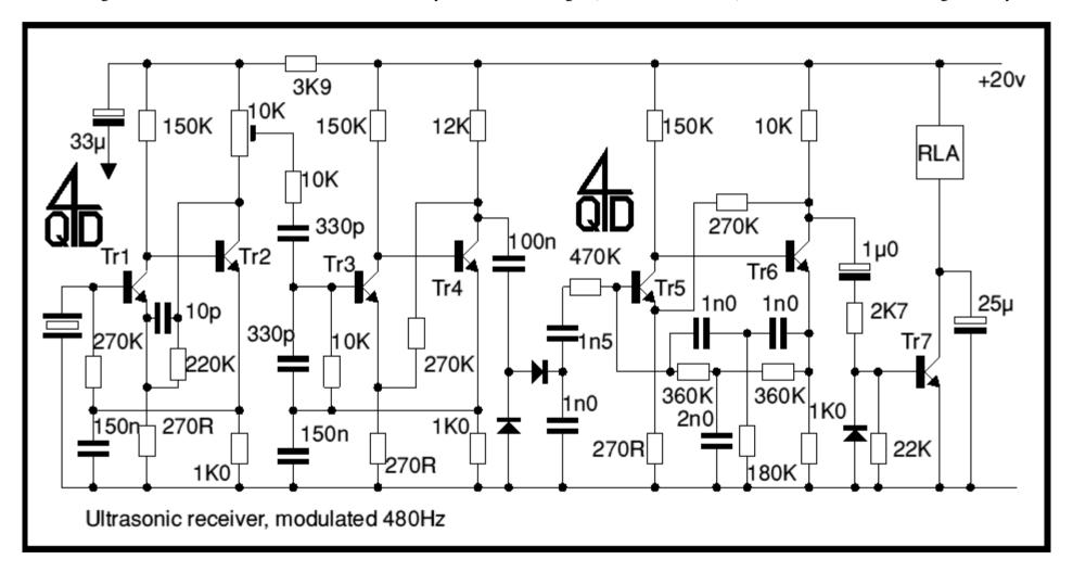
Stage 1 is the preamplifier: it is a fairly conventional circuit with gain fixed by feedback.
